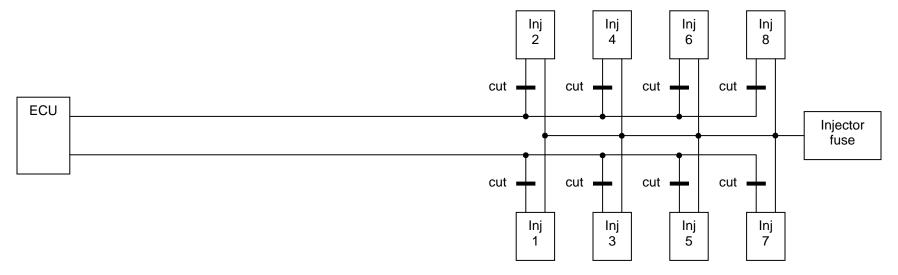
Step 2, identify the injector wire stubs (1a, 2a, 3a, etc, in the figure below) and the ECU stubs (1b, 2b, 3b, etc, in the figure below).
