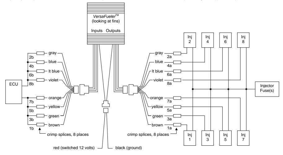
Step 4, attach the black wire ring terminal to a clean, shiny ground such as an engine or chassis bolt.
